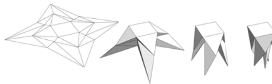
Figure 3: Discrete folding states of the optimized adapted flasher.
